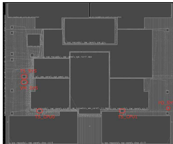
Figure 3: Placement of Synopsys temperature sensor, voltage monitor, and process detector IP within the Morello CPU architecture
